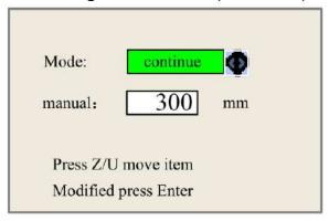
When the mode is set to "manual" pressing a direction button one time will cause the corresponding axis to move the designated distance.
