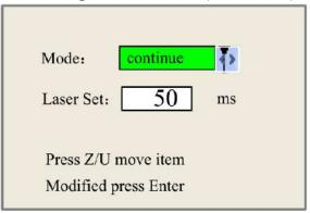
When the mode is set to "manual" pressing the Pulse button once will cause the laser to light for the designated time period.
