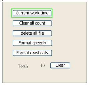
**CURRENT WORK TIME:** forecast current file's running time (accurate to 1ms)
