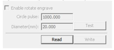
Click "Read" and RDwork will detect the rotary device.
