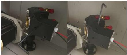
Repeat until the lasers are aligned properly.
