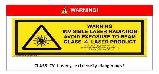
2. This machine is a CLASS IV laser device, which emits invisible radiation, and can be extremely dangerous.
