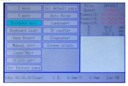
Press the "Z/U" button on the control panel, choose "Extended Axis", and then press "Enter" to access the secondary menu (as shown).
