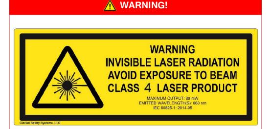
This machine is a Level 4 laser, which can cause serious permanent injury, including burned flesh and blindness.
