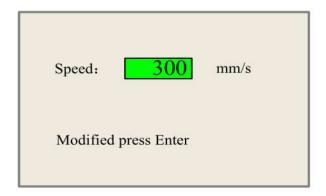
Push the "X+/-" buttons to move the cursor, and then push the "Y+/-" buttons to change the value.
