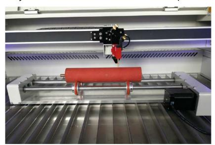
Plug the rotary device into the rotary port on the right side of the machine (as shown).
