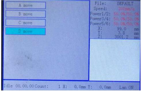
Select "D move", then the worktable can be moved up/down by pressing the arrow buttons.
