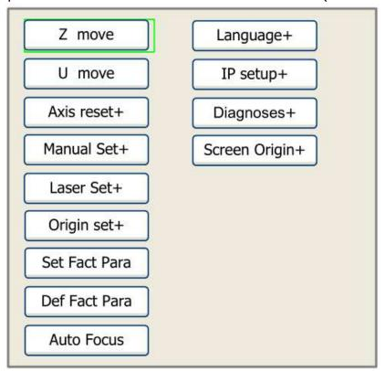
Push "Y+/-" buttons to move the cursor, and then press the "Enter" button to display the sub menu.
