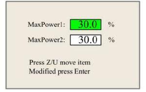
Pushing the "Z/U" button moves the cursor (green block), then "Y+/-" and "X+/-" buttons change the value.
