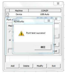
If the port test is unsuccessful, then power down the machine and computer. Restart and reattempt these Wi-Fi setup instruc-
