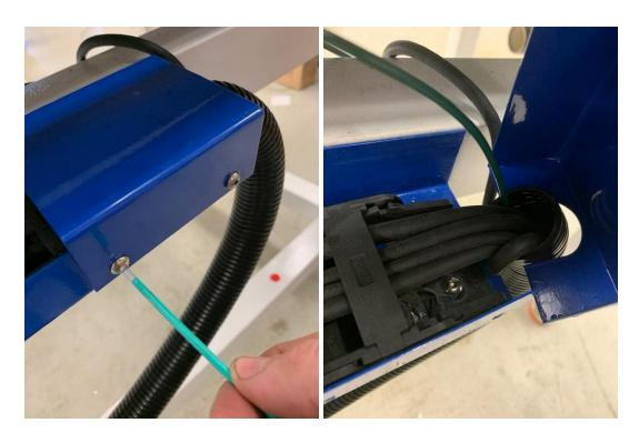
Once you have arrived at the connections find the calibrator connection and loosen all the screws on the connector.
