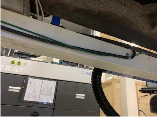
Once the wire has reached the track cable remove the cover and feed your wire through the loom back to the connections for the box. A wire fish may make this task easier, alternatively to this you may also bypass going through the loom and connect it externally to the loom via zip ties or electrical tape.
