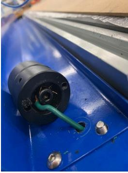
From here line up the threaded hole in the bottom of the calibrator with the bolt and tighten until snug. (please ensure once you have the bolt started in the thread rotate the calibrator as close to the machine bed as possible to allow for best contact with the calibrator puck.
