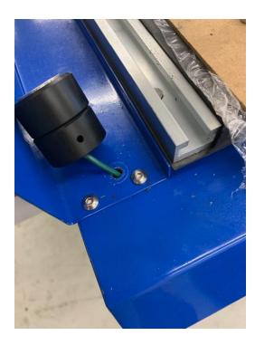
Take the bolt removed from the hole and after loosening the four side bolts holding on the front panel for better access (pictures below) insert the bolt back up through the hole from the underside of the front panel as shown in the second picture below.
