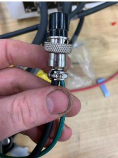
Once the nuts have been removed remove the metal cover to expose the wire connections. Please note you have to twist the plastic head to the right or counterclockwise before separating them.
